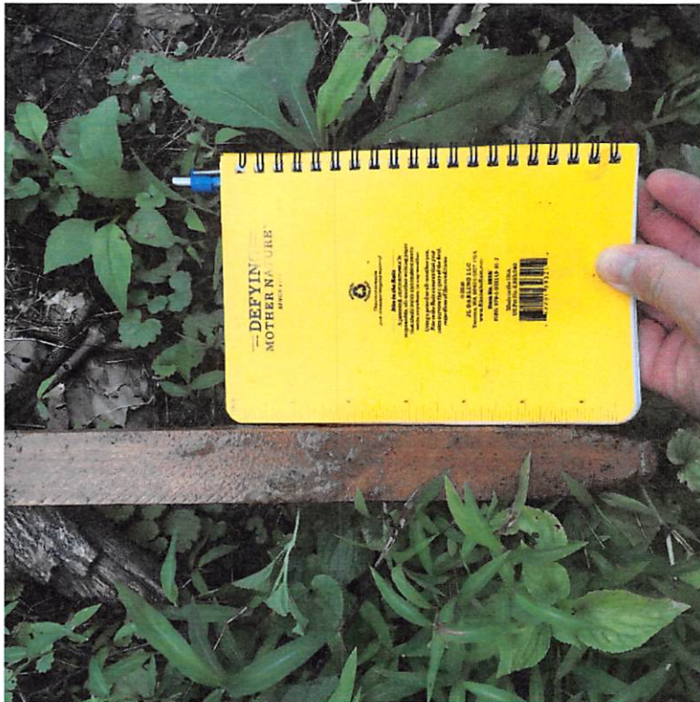
UNT of England's Run – In-stream sediment depth in excess of six inches (6") indicated by notebook.
